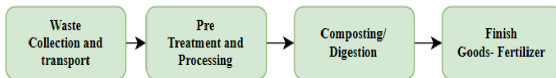
Figure 6: The cradle-to-gate system boundary defined for the life cycle assessment
